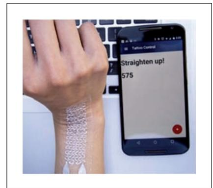
Figure 3. Skintillates are temporary tattoos that can do things. Pictured is a strain gauge warning the wearer to straighten her wrist. (Source: Joanne Lo; used with permission.)
