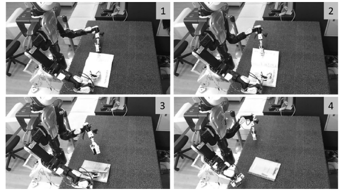
Fig. 10. Online generation test with untrained object: Book-closing test.
