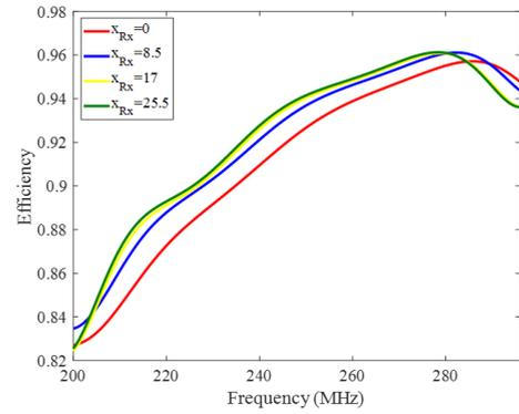
**FIGURE 4.** Efficiency of the system with respect to the position of the receiver over a wide frequency range (numerical results). The maximum efficiency occurs at 280 MHz (while the resonance frequency of a single Tx occurs at 250 MHz) due to strong coupling of our Rx with Tx1.
