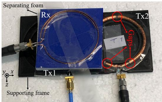
**FIGURE 2.** Picture of the fabricated system for experimental verification. Two transmitters are partially overlapped and fixed with a supporting frame. The space between the transmitters and receiver is filled by a separating foam that keeps the distance fixed during measurement.
