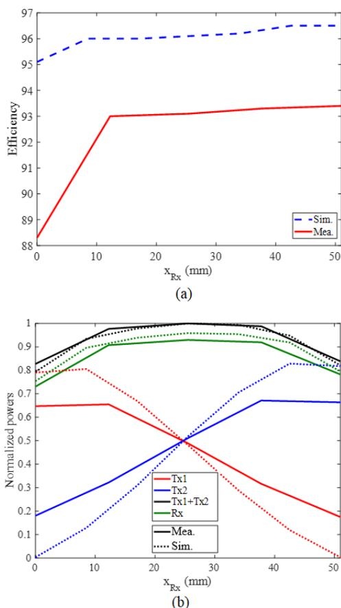
**FIGURE 5.** (a) Numerical and experimental results for the system efficiency with respect to the position of the receiver at frequency 280 MHz. (b) The powers delivered to the transmitters and the power received by the load normalized to the maximum total power extracted from the sources with respect to the position of the receiver. Solid lines represent the experimental results and dashed lines represent the numerical results.
