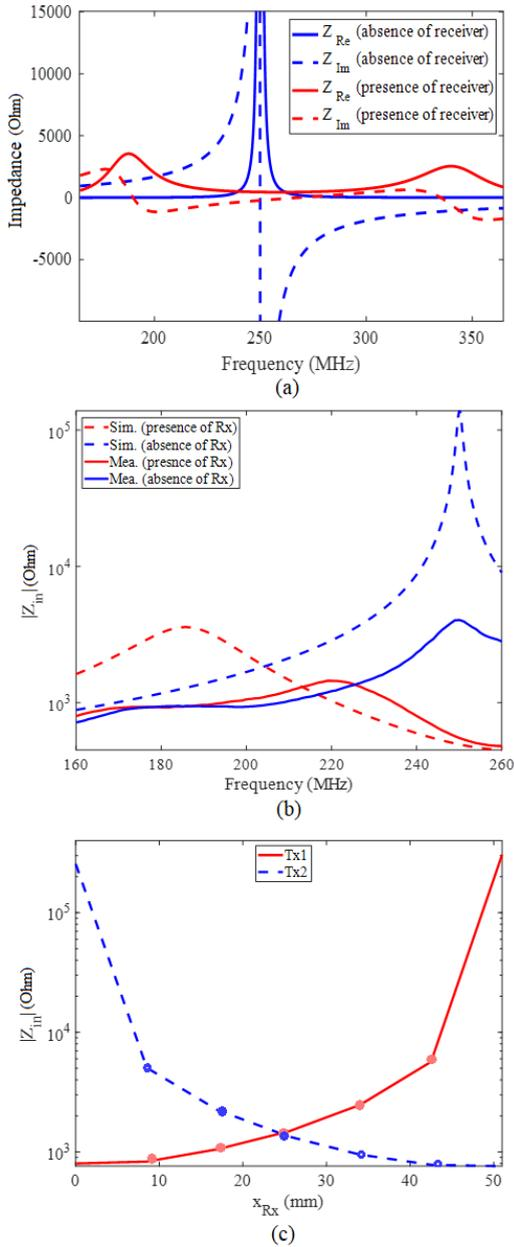
**FIGURE 3.** (a) Real and imaginary parts of the input impedance of the proposed transmitter in the absence and presence of the receiver (numerical results); (b) experimental results versus numerical ones for the absolute value of the input impedance. (c) The absolute values of the input impedances of both transmitters shown in Fig. 1(c) with respect to the receiver position (numerical results).
