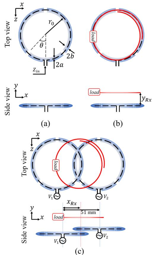
**FIGURE 1.** Schematic view of: (a) the proposed transmitter in free space, (b) the proposed transmitter in presence of the proposed receiver, and (c) the WPT system based on two overlapped transmitters and a receiver positioned above them.
