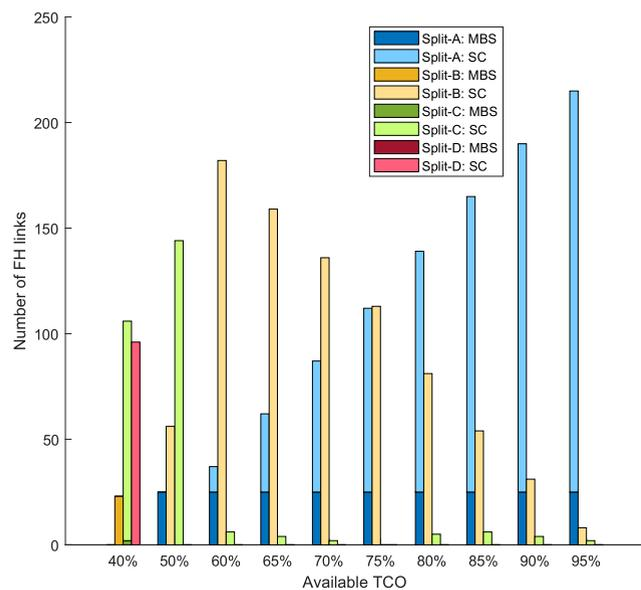
**FIGURE 12. Scenario 1, “fibre only” mode: Number of FH links utilizing different splits varying with different level of TCO availability - Maximizing centralization approach.**
