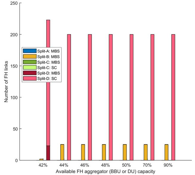
FIGURE 16. Scenario 2, “fibre only” mode: Revised number of FH links utilizing different splits varying with different level of capacity availability in BBU or DU - Minimizing TCO approach.
