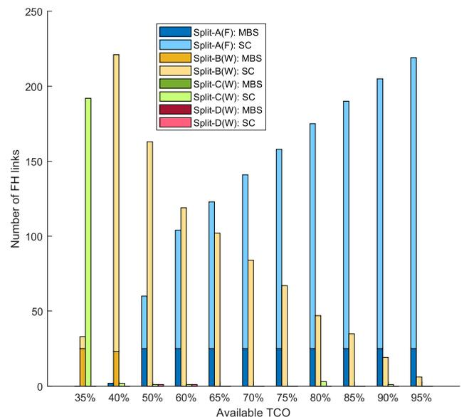
**FIGURE 13. Scenario 1, “heterogeneous” mode: Number of FH links utilizing different splits varying with different level of TCO availability - Maximizing centralization approach.**
