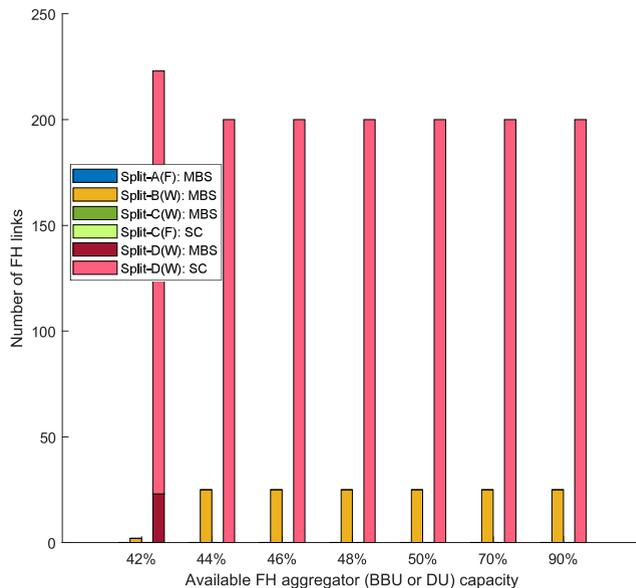
FIGURE 8. Scenario 2, “heterogeneous” mode: Number of FH links utilizing different splits varying with different level of capacity availability in BBU or DU - Minimizing TCO approach.
