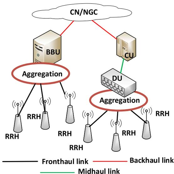
FIGURE 1. Heterogeneous transport network in 5G.
