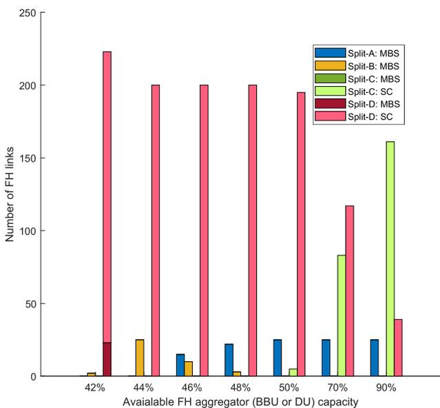
FIGURE 7. Scenario 2, “fibre only” mode: Number of FH links utilizing different splits varying with different level of capacity availability in BBU or DU - Minimizing TCO approach.
