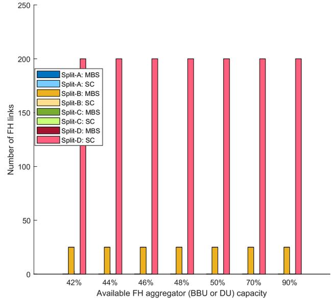
FIGURE 10. Scenario 1, “fibre only” mode: Revised combination of splits varying with different level of capacity availability in BBU or DU - Minimizing TCO approach.
