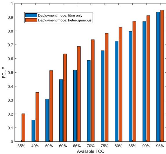
FIGURE 15. Scenario 1, FCUF comparison between the “fibre only” and the “heterogeneous” mode of deployments for the combinations presented in Fig. 12 and Fig. 13 - Maximizing centralization approach.
