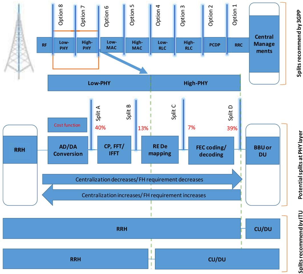
FIGURE 3. Potential splits at PHY layer and cost distribution.
