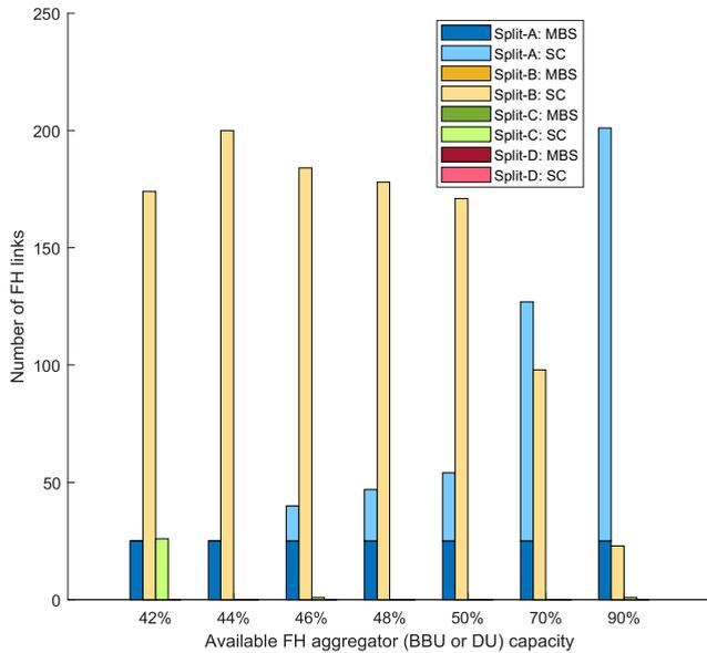
FIGURE 4. Scenario 1, “fibre only” mode: Number of FH links utilizing different splits varying with different level of capacity availability in BBU or DU - Minimizing TCO approach.
