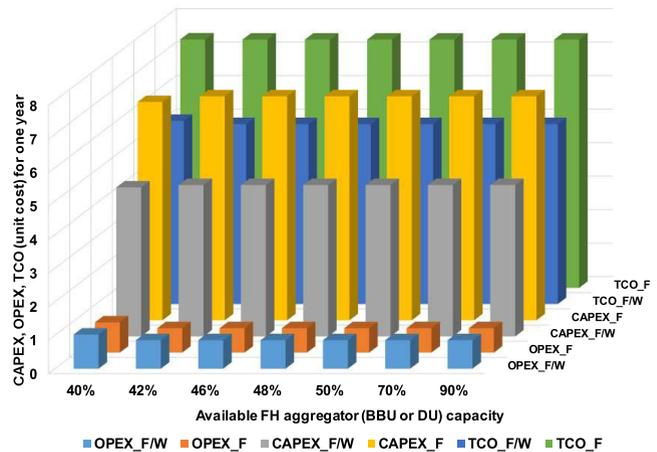
FIGURE 17. Scenario 2, Cost analysis of the optimal combinations for “fibre only” and “heterogeneous” mode - Minimizing TCO approach.
