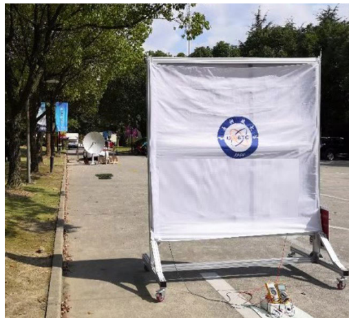
FIGURE 11. The Ku-band medium and long distance microwave wireless energy transmission system based on rectifier diode.
