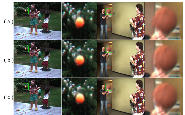
FIGURE 7. Examples of using different perceptual loss functions. (a) MPR + 3D U-net w/o any perceptual loss. (b) MPR + 3D U-net with original perceptual loss. (c) MPR + 3D U-net with multi-step perceptual loss.
