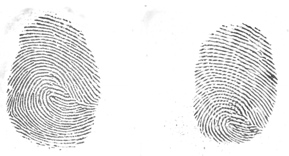
FIGURE 1. The left fingerprint is a live press fingerprint, whereas the right fingerprint is obtained by pressing a synthetic finger made out of wood-glue. The two fingerprints came from the same finger and so have matching identification [6] [2]. We aim to detect the liveness of the fingerprint press using a convolutional neural network.
