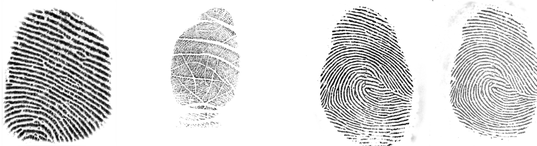
FIGURE 6. Examples of live fingerprints for Digital Persona, Crossmatch, Biometrika and Greenbit are shown in order from left to right.
