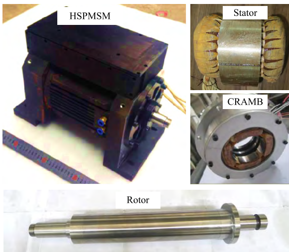
FIGURE 2. The HSPMSM and the major parts, such as stator, rotor and the CRAMB.
