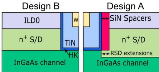
**FIGURE 3.** Schematic highlighting the implementation of spacers and RSD extensions in design A compared to design B.
