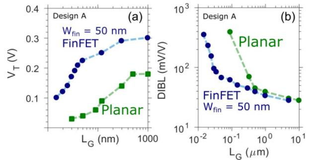
**FIGURE 9.** For design A, a)  $V_T$  versus  $L_G$  for planar (green) and FinFET (blue) devices with  $W_{fin} = 50$  nm showing  $V_T$  roll-off onset at  $L_G = 50$  nm. b) Drain-induce barrier lowering versus  $L_G$  for planar and FinFETs.
