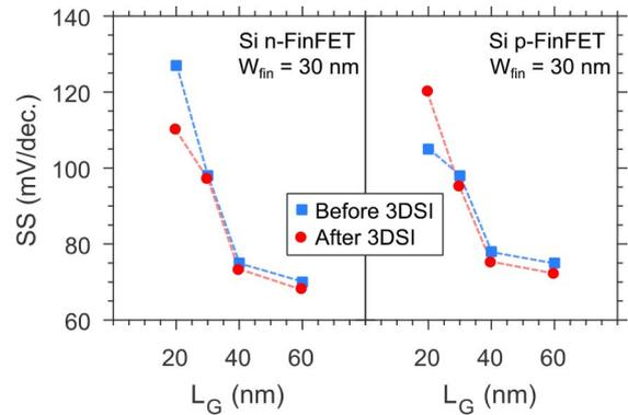
**FIGURE 5.** Subthreshold slope of Si CMOS n- and p-FinFETs in saturation, for devices with fin width of 30 nm before and after 3D sequential integration of the top III-V transistor level. Negligible change of SS is observed as a result of the 3DS integration.
