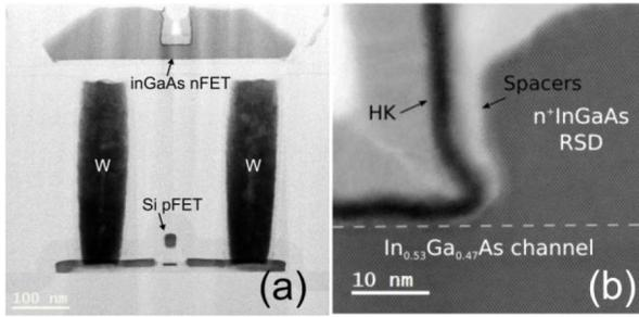
**FIGURE 2.** a) STEM cross-section of the 3DS integrated stack showing both transistor levels. Cross-section along the gate showing an InGaAs nFET with  $L_G = 60$  nm on top of a Si pFET.  $W$  inter-layer contacts are also shown. b) Detailed STEM image of the InGaAs FET gate region featuring design A. High crystalline quality for the InGaAs channel is shown. The  $\text{Al}_2\text{O}_3/\text{HfO}_2$  gate oxide and the approximately 4 nm thick  $\text{SiN}_x$  spacers are highlighted.
