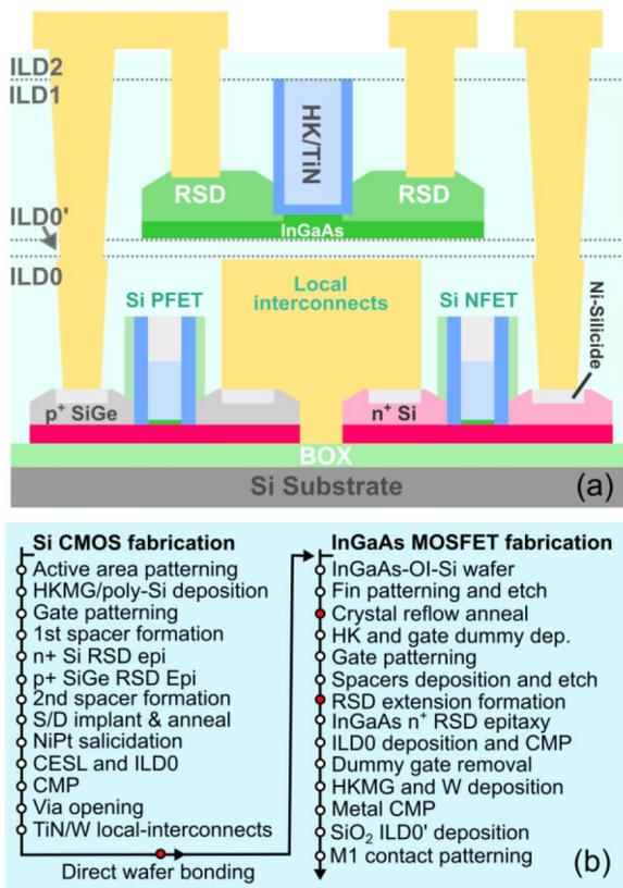
**FIGURE 1.** On top, schematic of the 3DS integrated stack, InGaAs nFETs on top of fully-depleted silicon-on-insulator Si pFETs and nFETs. A gate-first process is used for the Si CMOS and a RMG process for the InGaAs nFETs. Below, process flow schematic for the Si CMOS gate-first fabrication (left) and InGaAs nFET fabrication (right). Red dots indicate new or improved process modules in this work.
