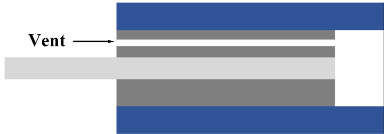
Fig. 2. An extrinsic FPI pressure sensor with a vent.
