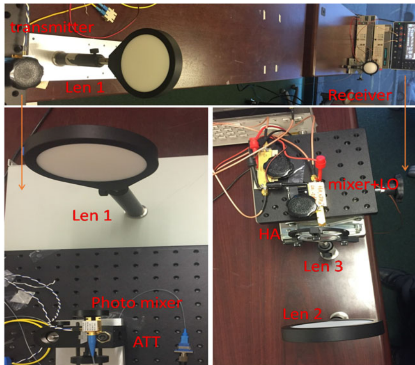
Fig. 3. Picture of the experimental setup for fiber-wireless-fiber integration transmission system at THz-band.
