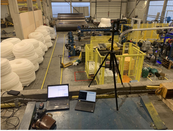
Fig. 2. Industrial site at Krah Pipes OÜ, which manufactures thermoplastic pipes in a complex industrial environment. The site contained a network of eight UWB anchors (layout in Fig. 19).
