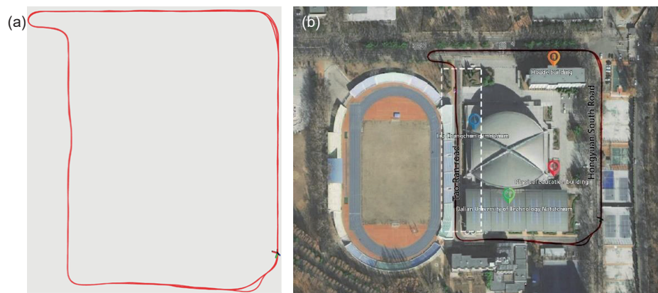
Fig. 16 Matching effect of trajectory based on the Lidar-IMU-Camera system and satellite map. (a) Trajectory information based on the Lidar-IMU-Camera system; (b) trajectory matching result related to the satellite map.
