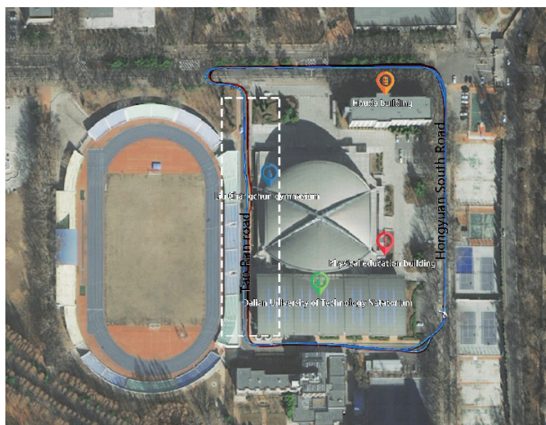
Fig. 17 Trajectory comparison between the Lidar-IMU-Camera and the LEGO-LOAM systems.
