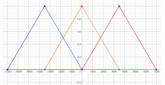
Fig. 3. Graphical representation of the membership functions of the fuzzy logic-based active controller.
