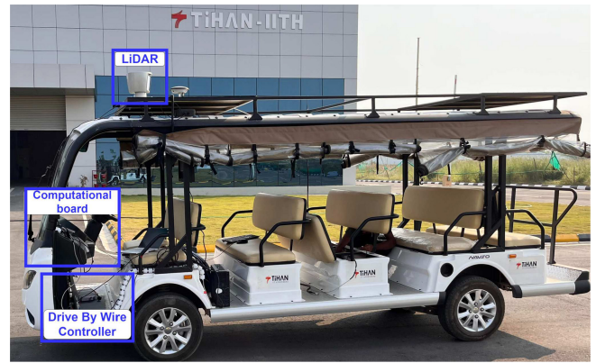
FIGURE 2. E-vehicle mounted with Velodyne HDL-64 LiDAR, NVIDIA Jetson AGX Orin computing platform, and MicroAutoBox vehicle controller.
