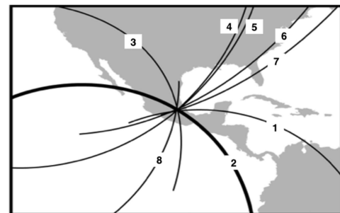
FIGURE 2. Example of individual SMLS scan swaths on successive orbits. In this example, the atmosphere over Mexico City is repeatedly observed on 8 successive orbits. The orbits are numbered sequentially, with orbit number 2 (shown with a thicker line) being the orbit shown in Fig. 1.
