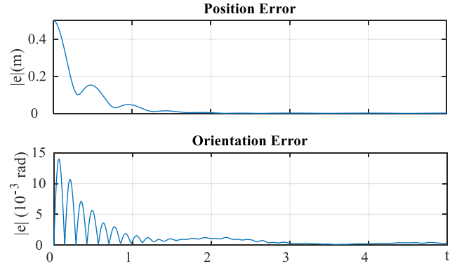
Fig. 17. Position and orientation error of the EE tracking the sinusoidal trajectory from Fig. 16.
