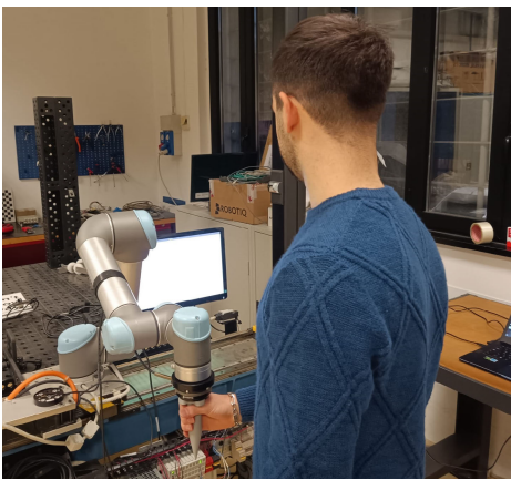
Fig. 6. Experimental setup: a Robotiq FT300 sensor is at the robot tip; a monitor shows the reference trajectory.
