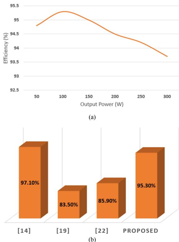
**FIGURE 13.** (a) Experimental efficiency of the proposed converter, (b) Experimental efficiency comparison of the converters at 100 W output power.
