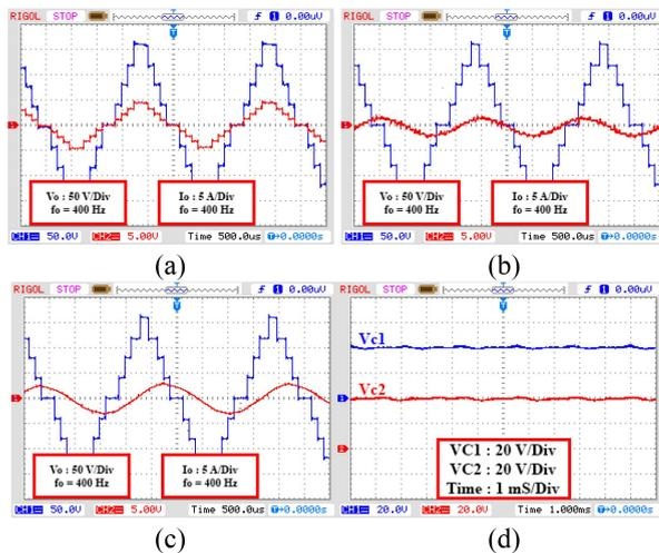
FIGURE 10. Experimental results of output voltage and current at (a) resistance load ( $R$ ), (b) resistance inductance load ( $35\Omega + 5\text{ mH}$ ) and modulation index of 89%, (c) resistance inductance load ( $35\Omega + 60\text{ mH}$ ) and modulation index of 80%, and (d) capacitors voltage.
