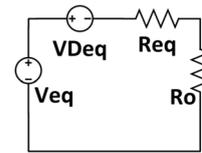
**FIGURE 5.** Equivalent current path.
