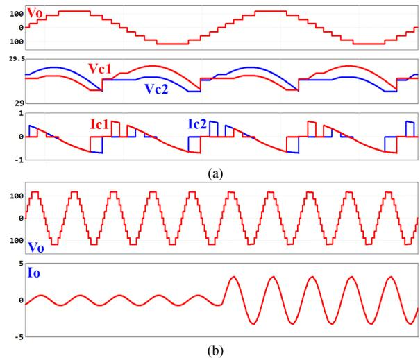
**FIGURE 8.** Simulation waveforms of (a) output voltage and capacitor voltages and currents, (b) output voltage and output current under load change.
