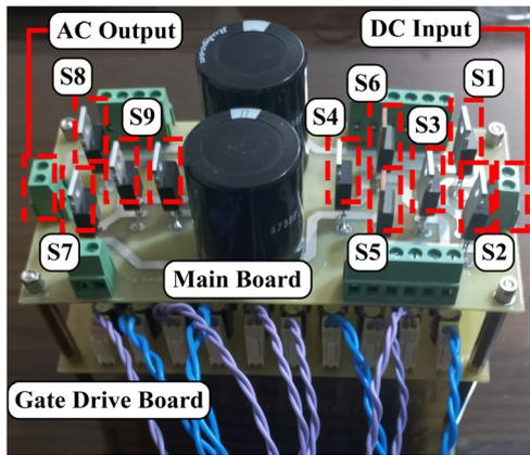
FIGURE 9. Experimental setup.
