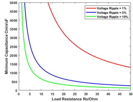
**FIGURE 4.** Load resistance versus minimum capacitance at the frequency of 400 Hz.
