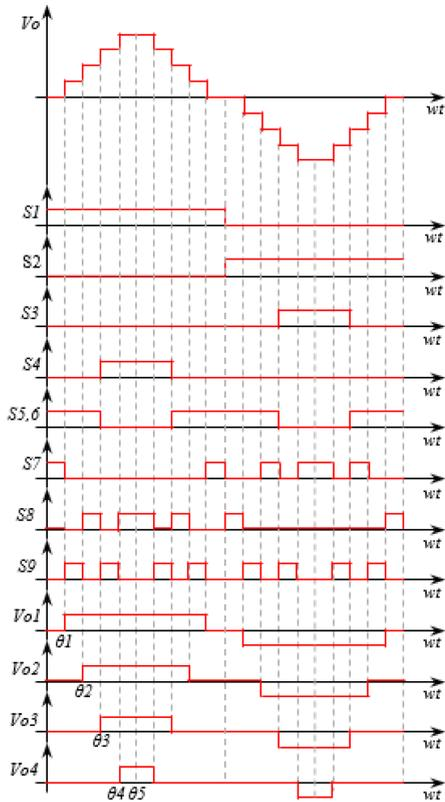
**FIGURE 3.** Switching patterns and the output voltage at each voltage level.
