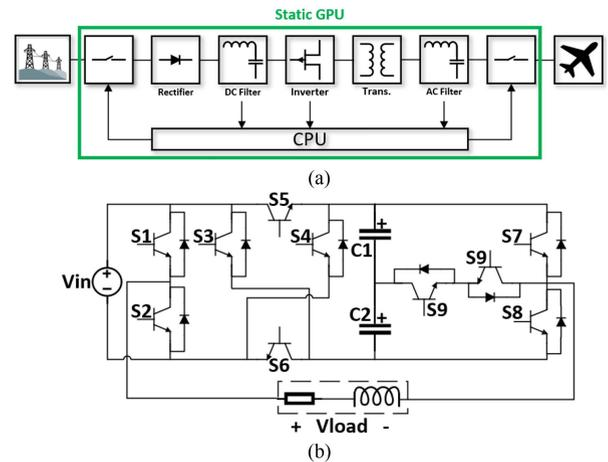
FIGURE 1. (a) Schematic diagram of static ground power unit, (b) Proposed circuit topology of the nine-level inverter.
