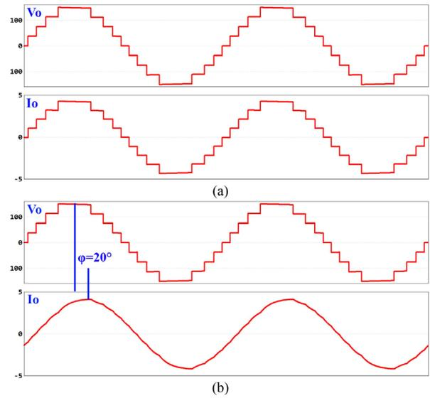
**FIGURE 7.** Simulation results of output voltages and currents under different load types. (a)  $R_o = 35 \Omega$ . (b)  $Z_L = 35 \Omega + j12.5$  ( $R_o = 35 \Omega$ ,  $L_o = 5 \text{ mH}$ ,  $\varphi = 20^\circ$ ).
