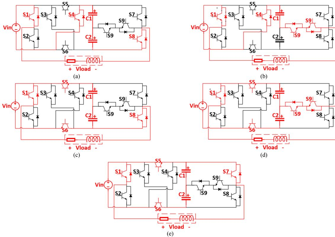
FIGURE 2. Switching patterns at the level of (a)  $2V_{DC}$ , (b)  $1.5V_{DC}$ , (c)  $V_{DC}$ , (d)  $0.5V_{DC}$ , (e)  $0^+$ .
