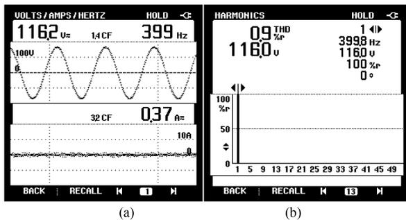
**FIGURE 12.** Experimental waveforms of (a) Output voltage, (b) Total harmonic distortion (THD).
