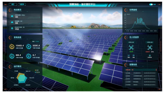
FIGURE 7. Interface of a data-driven simulation digital twin model of a solar farm [86].
