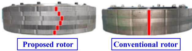
FIGURE 35. Rotors with step herringbone skew (left) and without skew (right) [73].
