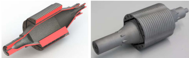
FIGURE 31. Sectional view of CAD model (left) and photograph of functional model after production (right) [65].
