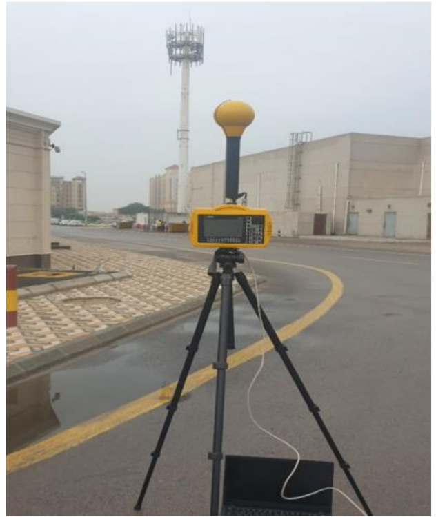
FIGURE 8. The measurement location where the radiation meter is placed in front of the antennas for the multi-technology site.
