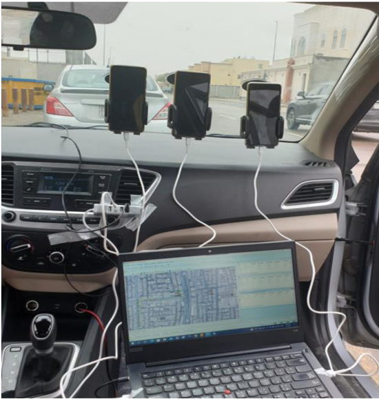
FIGURE 10. The tool setup for field drive test measurements.
