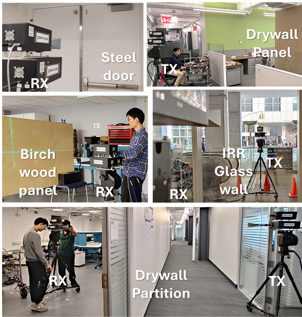
FIGURE 9. Panels of different MUTs, such as drywall and wood were measured in a lab setup, whereas partitions, such as IRR glass walls required TX and RX set up on both sides of the MUT.
