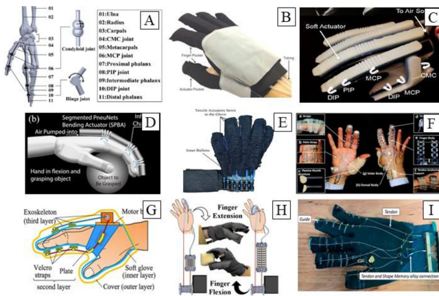
Fig. 10. Hand exosuits. A) Hand anatomy: Joints and bones, B, C, D, E) Pneumatically actuated hand assistive device [98]– [101], F, G, H) Cable driven assistive gloves, [102], [103], [104] D) SMA actuated assistive glove for finger flexion/extension [105].
