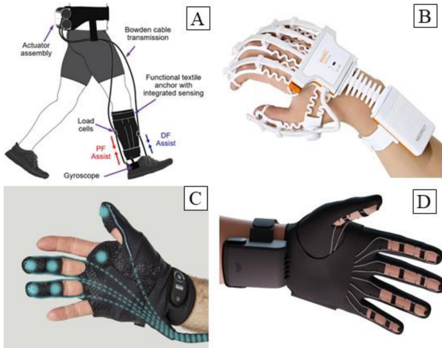
Fig. 16. Commercially available exosuits: A) ReWalk Robotics ReStore [207], B) Neofect smart glove [208] C) carbon hand [209], D) NUADA glove [210]
