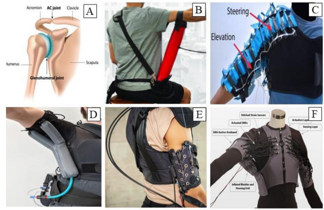
Fig. 7. Shoulder exosuits. A) Shoulder anatomy: Joints and bones, B) Exomuscle: Reel type pneumatic actuator [46], C) Pneumatically actuated soft exosuit to assist the shoulder movement [47], D) An inflatable pneumatic exosuit to support the shoulder against the gravity [48], E) A cable driven exosuit for shoulder movement in 3D space [49], E) A hybrid pneumatic and SMA based exosuit for shoulder [50].
