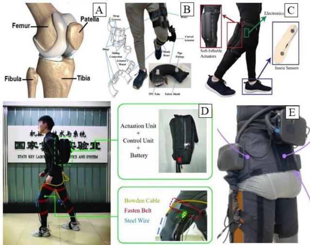
Fig. 13. Knee exosuits: A) Knee anatomy: Joints and Bones, B, C) Pneumatically actuated knee exosuit [166], [167], D) Cable driven knee exosuit [168], E) Cable driven knee abduction movement assistance exosuit [169].
