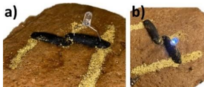
Fig. 3. Voltage divider: a) After fabrication; b) In operation regime.
