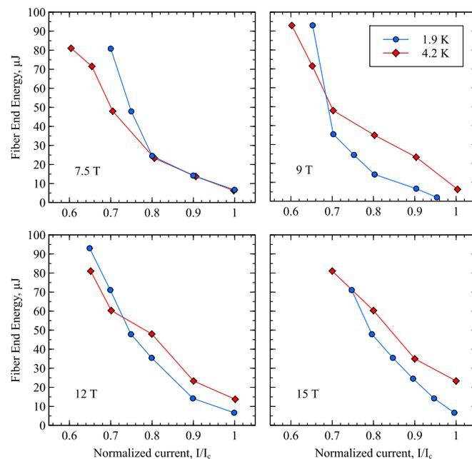
**Fig. 6.** The energy required to induce a quench of the RRP@ wire vs. normalized current at 1.9 K and 4.2 K at selected magnetic field levels.
