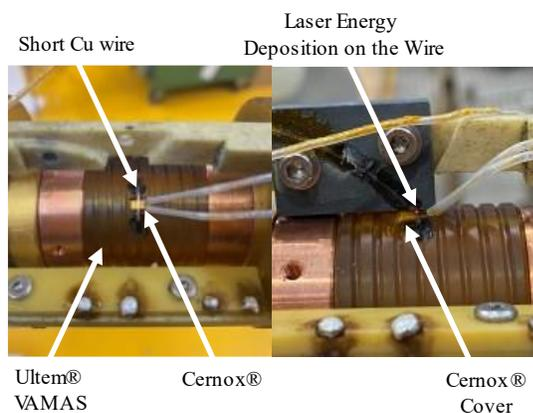
**Fig. 2.** Calibration setup with a short copper wire installed over a Cernox® temperature sensor.
