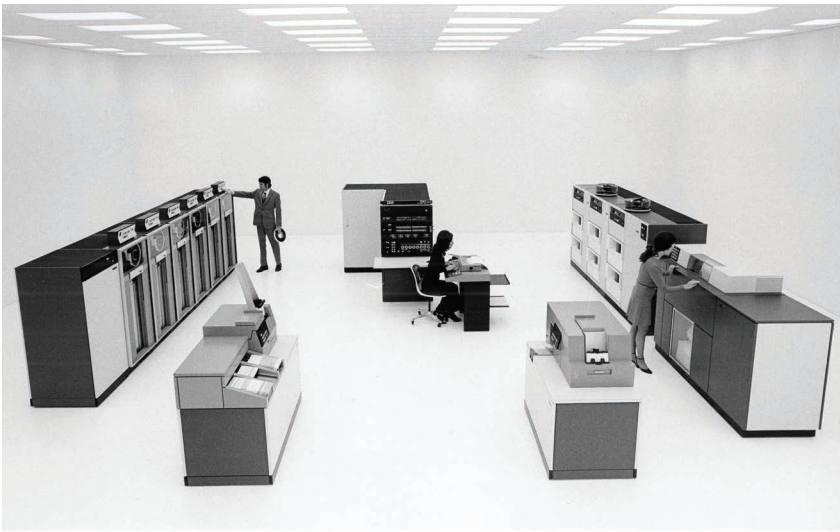
FIGURE 5. The 1970 System 370 Model 145 was the first IBM computer with all the major memory elements fabricated on a single silicon chip. It marked IBM's first move away from the magnetic-ferrite-core technology that had been the mainstay of computer memory since the mid-1950s. Six months after the announcement of the System 370, the nickname Silicon Valley appeared in print for the first time in an issue of Electronic News . The era of silicon had begun. (Reprint courtesy of IBM Corporation ©.)
