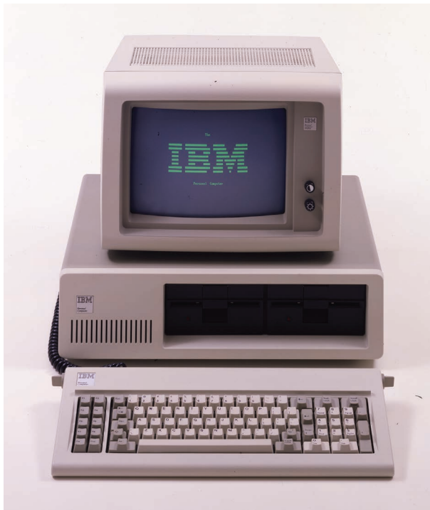
FIGURE 8. Introduced in 1981, the IBM 5150 was IBM's first PC to use the Intel 8088 microprocessor. (Reprint courtesy of IBM Corporation ©.)
