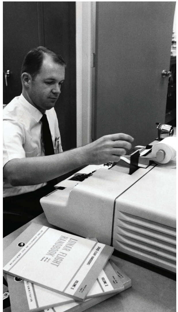
FIGURE 3. A NASA scientist works with the Olivetti P101 (1969). The P101 was used as a calculation tool for the Apollo 11 mission in preparation for the various phases of the journey, from the compilation of lunar maps to the choice of moon landing location and the trajectory of the journey. (Courtesy of Associazione Archivio Storico Olivetti, Ivrea—Italy. Used with permission.)
