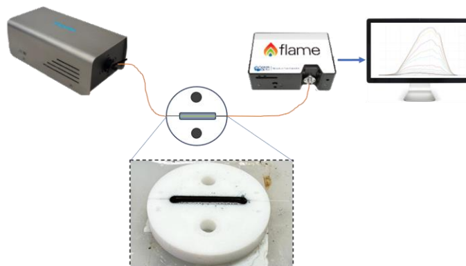
Fig. 3. Experimental setup of the novel fiber-optic pH sensor.
