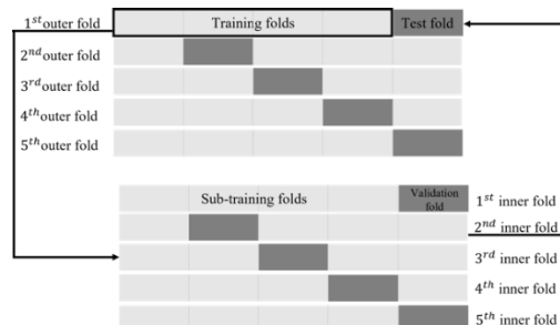
Fig. 6. Nested cross validation. Split the data (90% of the entire dataset) into K outer folds ( K = 5 as example). Then, all the K-1 folds are merged and split into inner folds (5 inner folds as example). Feature selection and training are performed using the inner sub-training folds, and testing is performed on the remaining inner fold. Use the best inner training model including features extracted for train the classification model on the entire outer training dataset and test on the outer testing fold.
