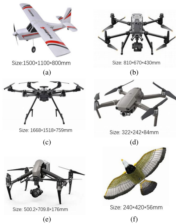
Fig. 13. Types of drones and bionic bird. (a) Fixed wing drone. (b) DJI M350. (c) Hexacopter. (d) DJI Mavic2. (e) DJI Inspire2. (f) Bionic bird.
