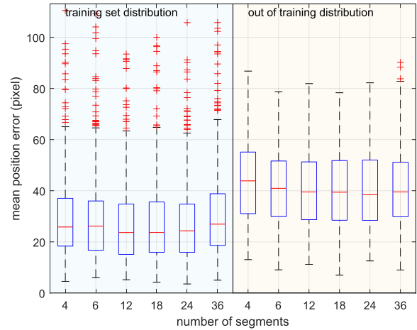
Fig. 11. Reconstruction error as a function of the number of segments for the complex model. (L) Training set distribution = ID set. (R) Out of training distribution = OOD set.
