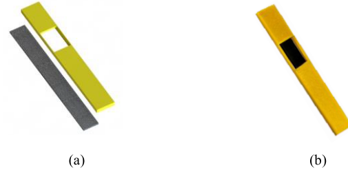
Fig. 5. Sample with template aid. (a) Three-dimensional model and (b) real model.
