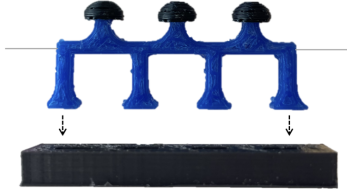
Fig. 7. Photograph of the final prototype, including the base, body structure, and contact heads.
