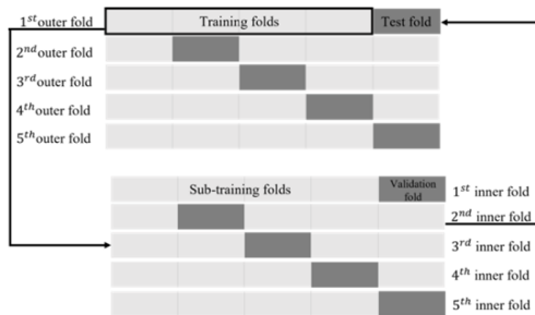
Fig. 6. Nested CV. Split the data (90% of the entire dataset) into K outer folds ( K = 5 as an example). Then, all the K - 1 folds are merged and split into inner folds (five inner folds for example). Feature selection and training are performed using the inner subtraining folds, and testing is performed on the remaining inner fold. Use the best inner training model, including features extracted to train the classification model on the entire outer training dataset and test on the outer testing fold.
