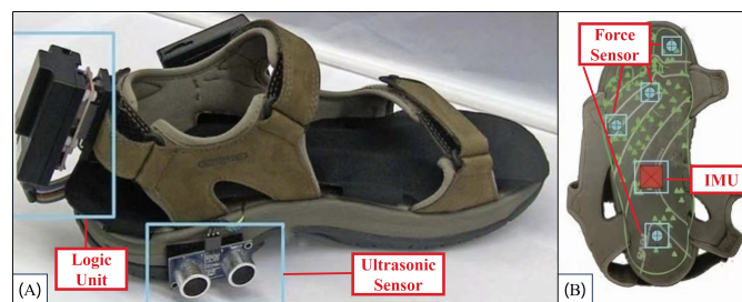
Fig. 1: The instrumented footwear (i.e., SoleSound ) used in this study [34]. (A) The logic unit is attached to the heel, and the ultrasonic sensor is mounted on the medial side of the footwear, although it was not used in this study. (B) The locations of the four piezoresistive force sensors and the 9-DOF IMU.
