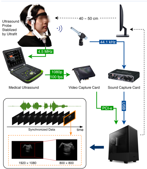
Fig. 1. Experimental system for audio and ultrasound tongue image acquisition and image preprocessing. The green line represents the acquisition process of ultrasound tongue images, while the blue line represents the audio acquisition process. Image preprocessing is depicted within the black frame.
