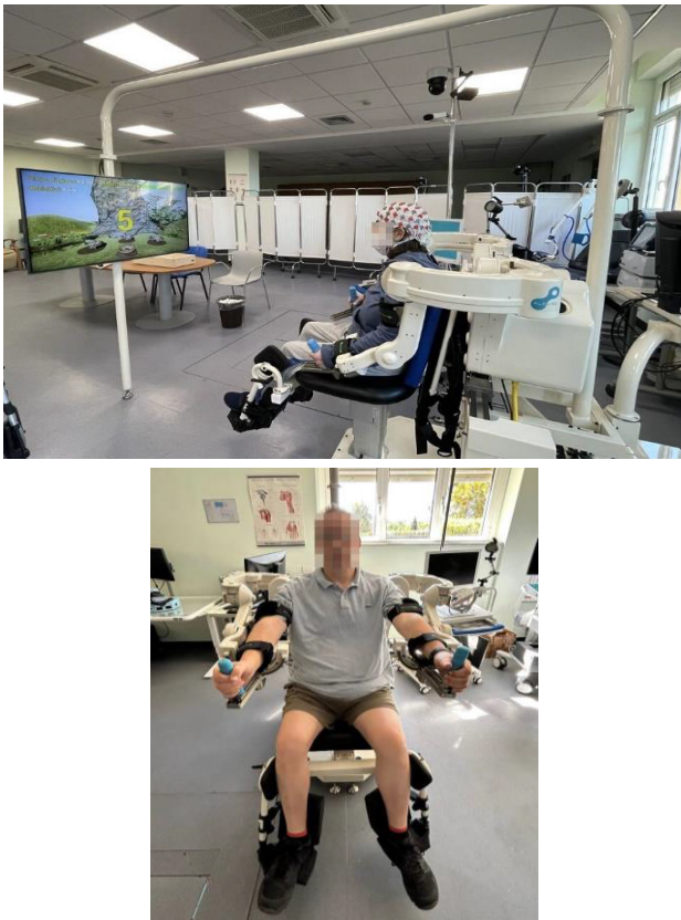
Fig. 1. Arm Light Exoskeleton Rehab Station (ALEX RS). Lateral (top) and frontal view (bottom).
