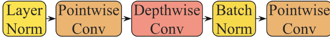
Fig. 4. The detailed structure of the convolution module used in the conformer blocks.
