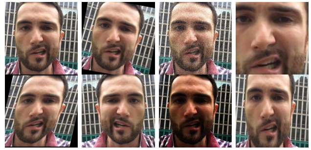
Fig. 4. Illustration of the dataset augmentation over a sample image. The images of each row from left to right: raw image, rotating, adding noise, cropping, shearing, flipping, brightness, and scaling.
