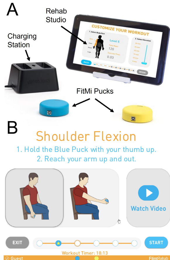
Fig. 1. Description of the FitMi system. A) FitMi system consists of 2 force and motion-sensing pucks, a charging station, and RehabStudio (a software application for gamified exercise). B) An example of an arm exercise (i.e., shoulder flexion exercise) that is shown in RehabStudio.
