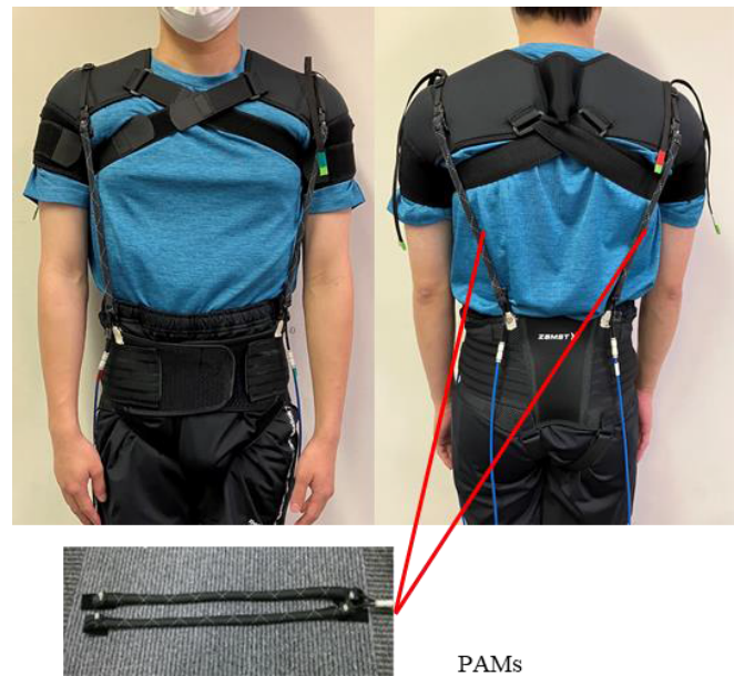
Fig. 1. Wearable balance training device (WBTD). Lateral PAMs were used for unexpected perturbation.
