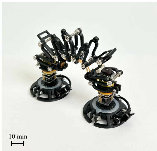
Fig. 1. Steerable flipping elastic robot. The total weight is 54 g. The weight near the end point of the body (motor + gripper) is 20 g.
