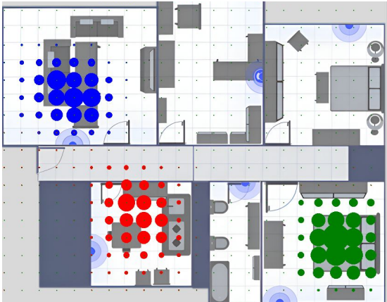
Fig. 3. Localisation heatmap of the 3 users involved in the dataset where they are located in the kitchen, livingroom and bedroom (07/25 15:13:00).
