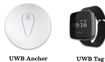
Fig. 2. Overview of UWB devices deployed for indoor location of individuals within the environment. The deployment uses anchors and wearable UWB tags (wristwatches) assigned to each resident.
