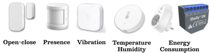
Fig. 1. Overview of ambient sensors deployed in the environment for capturing user interactions with household elements, such as door status, temperature, humidity, presence, motion, and power consumption.
