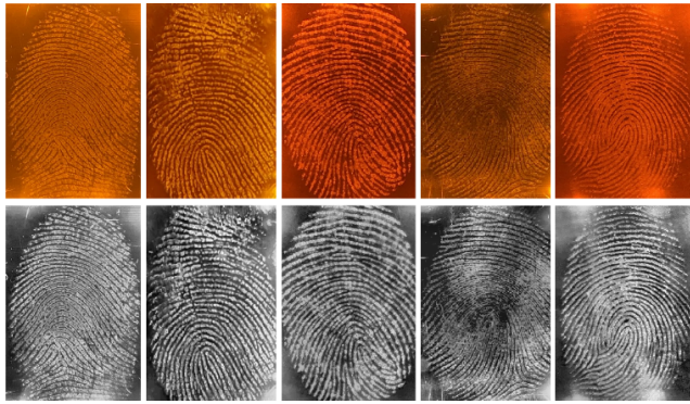
FIGURE 6. Acquired trace samples with the developed apparatus and normalization results with CLAHE
