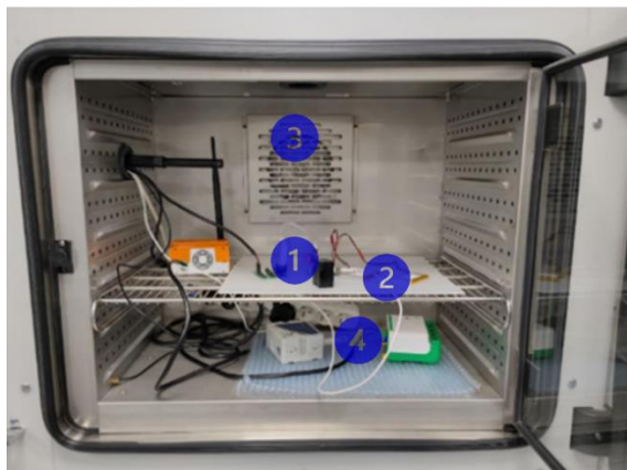
FIGURE 4. Temperature and humidity sensors characterization in a climatic chamber (● Smile device, ● battery, ● climatic chamber and ● reference instrument).
