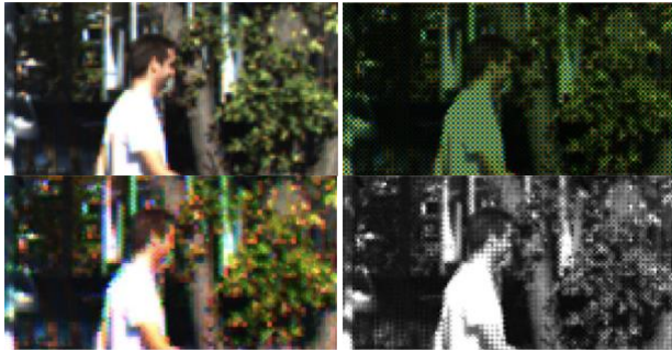
Fig. 4. Original detail from a KITTI frame top left, Bayer 0-Filled frame top right, Bayer Colour-Filled bottom left and single channel gray Bayer bottom right.
