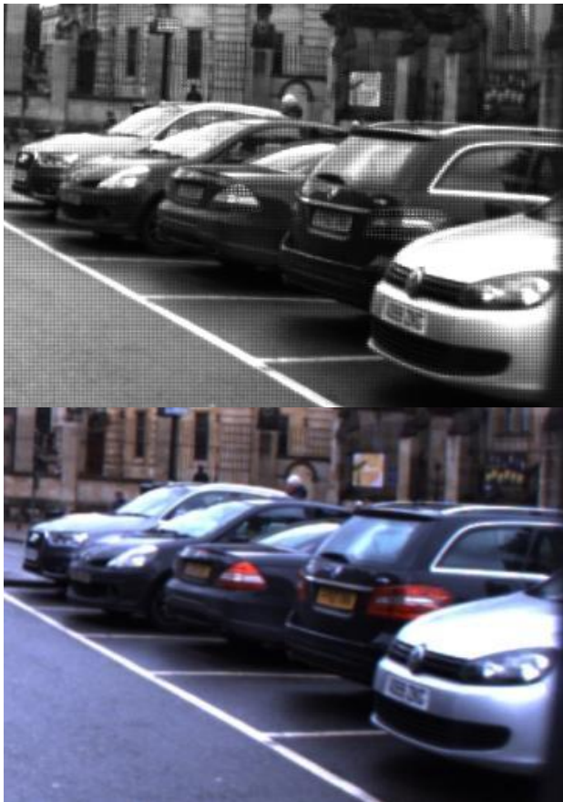
Fig. 1. A frame from the Oxford Robocar dataset [17]. Top is the raw frame from the dataset, bottom is the same frame after ISP processing and conversion in 3 colour channels.
