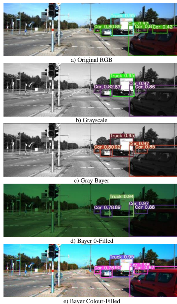
Fig. 8. Objects detected by the trained network overlaid onto the frame 000400.png. The training and evaluating dataset uses the same frame formats
