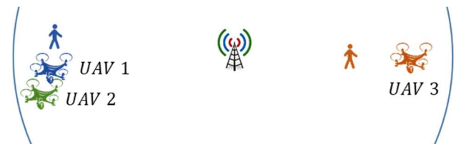
Figure 6. Depicts configurations which may cause collision between UAVBS 1 and UAVBS 2 and a quasi-equilibrium for UAVBS 3.
