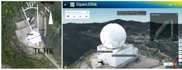
FIGURE 2. The size of the obstruction (left panel) and the relationship of the obstruction (right panel) [36]. In the left panel, the yellow point notifies the receiver. And the azimuth of the center of the obstruction is 330°. We assume the obstruction is a sphere. According to the measurement tools, the diameter of the sphere is about 14 m, and the horizontal distance from the center of the sphere to the receiver is about 10 m, the height difference between the top of the sphere and the receiver is about 11 m.
