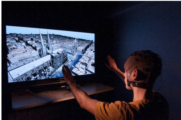
FIGURE 5. Illustration of a BCI being used to monitor User eXperience (UX) from EEG signals to assess and adapt 3D interaction tasks accordingly (©Inria / Photo H. Raguet).
