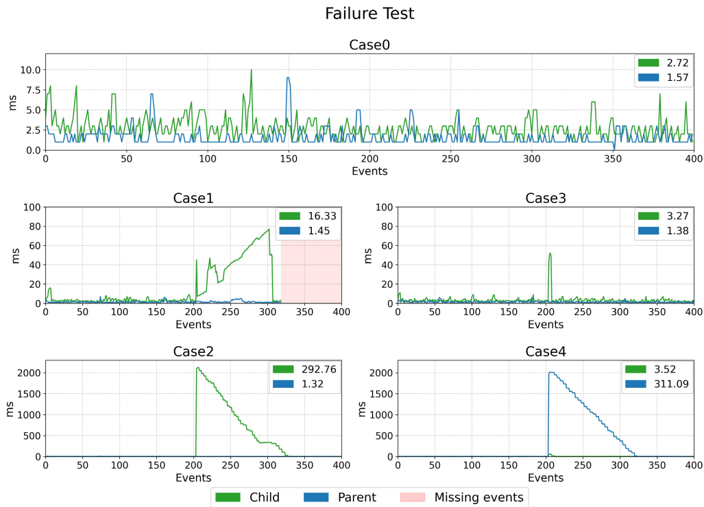
FIGURE 10. Failure Test results showing per-app processing latency for each event of a continuous stream generated by a 50x topology. Halfway through this event stream (200th event), an ONOS instance handling an application component is killed. This forces the missing functionality leadership to migrate to the other active cluster instance. Case0 represents the baseline with no failure. Case1 and Case2 kill an ONOS instance on the child cluster C1 handling one of the HSC application components, EventListener and EventSender respectively. Case3 and Case4 do the same, but on the parent cluster P running HSP’s EventReceiver and EventPublisher components.
